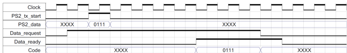
Fig. 10: Timing waveform for one cycle, sending data value 0111 from the PS/2 interface to your Synthesizer.
