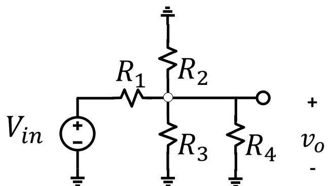
$$v_o = \frac{R_2 \parallel R_3 \parallel R_4}{R_1 + (R_2 \parallel R_3 \parallel R_4)} V_{in}$$
