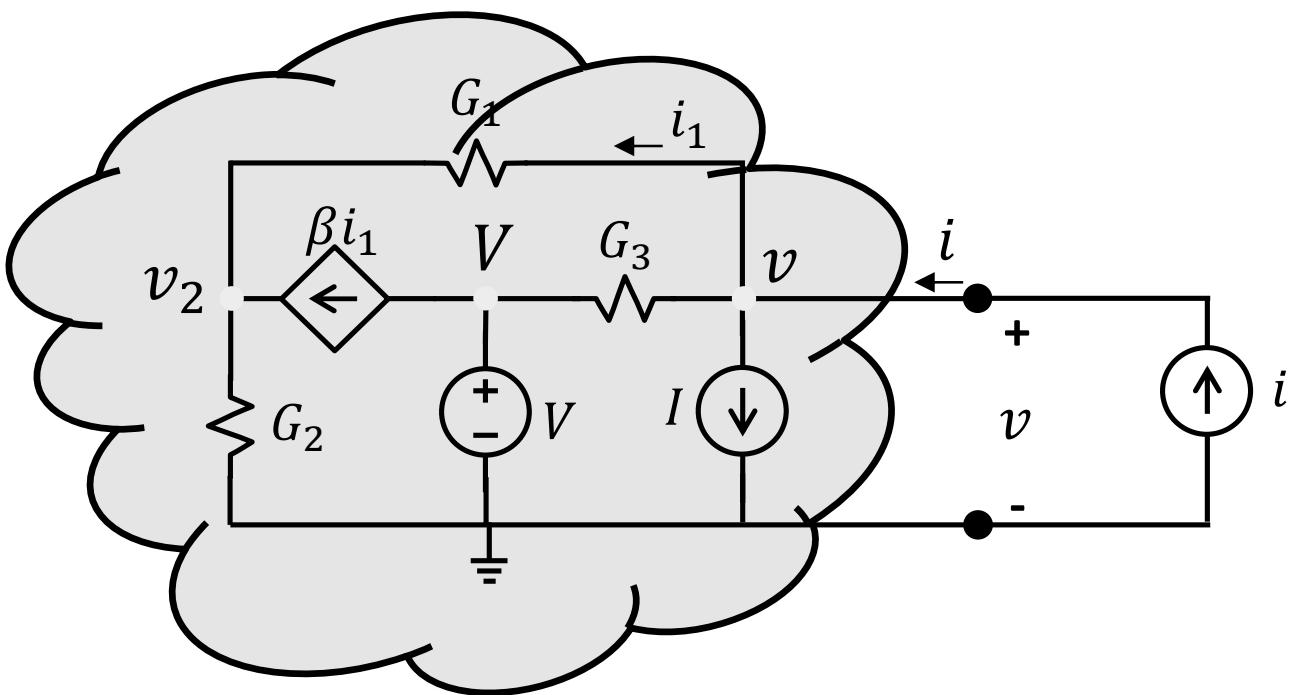
$$\begin{cases} \boxed{v}: & G_1(v - v_2) + G_3(v - V) + I - i = 0 \\ \boxed{v_2}: & G_1(v_2 - v) + G_2 v_2 - \beta G_1(v - v_2) = 0 \end{cases}$$
