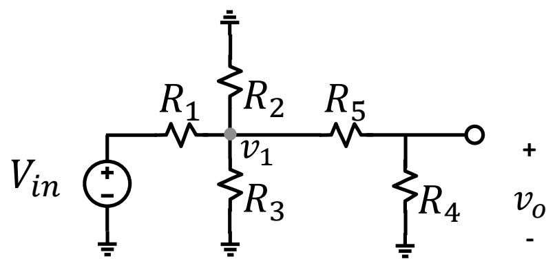
$$v_1 = \frac{R_2 \parallel R_3 \parallel (R_4 + R_5)}{R_1 + (R_2 \parallel R_3 \parallel (R_4 + R_5))} V_{in}$$
