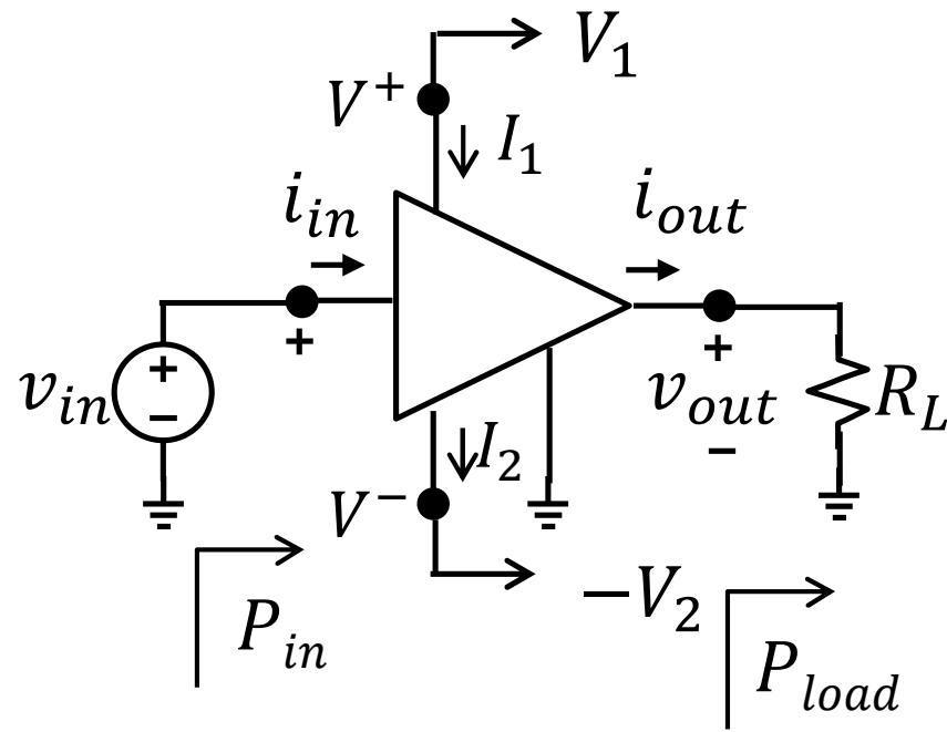
$$\left\{ \begin{array}{l} V_{1,2} = \pm 10V \\ I_1 = 9.5mA \quad I_2 = 9.5mA \\ v_{in} = 1^V \sin \omega t \quad v_{out} = 9^V \sin \omega t \\ i_{in} = 0.1^{mA} \sin \omega t \quad R_L = 1^{k\Omega} \end{array} \right.$$
