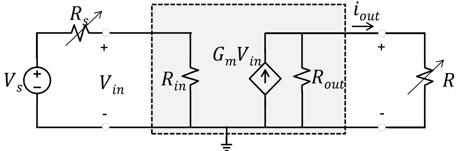
Short circuit:  $R_L = 0 \rightarrow \frac{i_{out}}{V_{in}} = G_m \quad \left[ \frac{A}{V} = \Omega^{-1} \right]$  short circuit Trans-conductance
