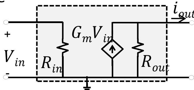
$$G_m = \frac{i_{out}}{V_{in}} \Big|_{V_{out}=0}$$
