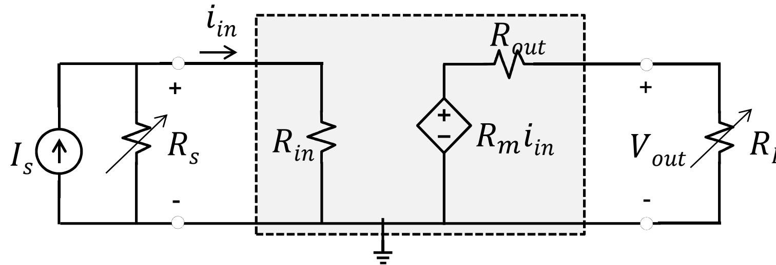
Short circuit:  $R_L = \infty \rightarrow \frac{V_{out}}{i_{in}} = R_m \quad \left[ \frac{V}{A} = \Omega \right]$  open circuit Trans-resistance
