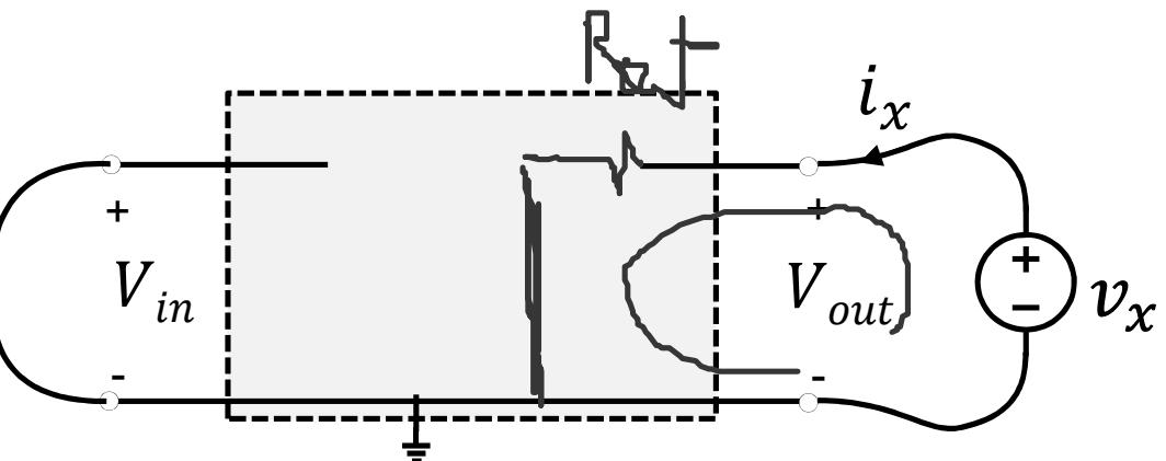
$$R_{out} = \left. \frac{v_x}{i_x} \right|_{V_{in}=0}$$
