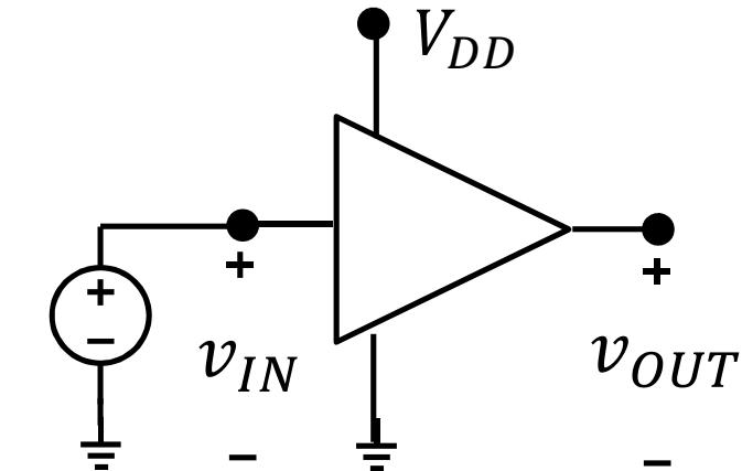
Open circuit:  $R_L = \infty \rightarrow \frac{V_{out}}{V_{in}} = A_{VO} \quad \left[ \frac{V}{V} \right]$  open circuit voltage gain
