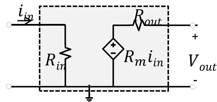
$$R_m = \frac{V_{out}}{i_{in}} \Big|_{i_{out}=0}$$
