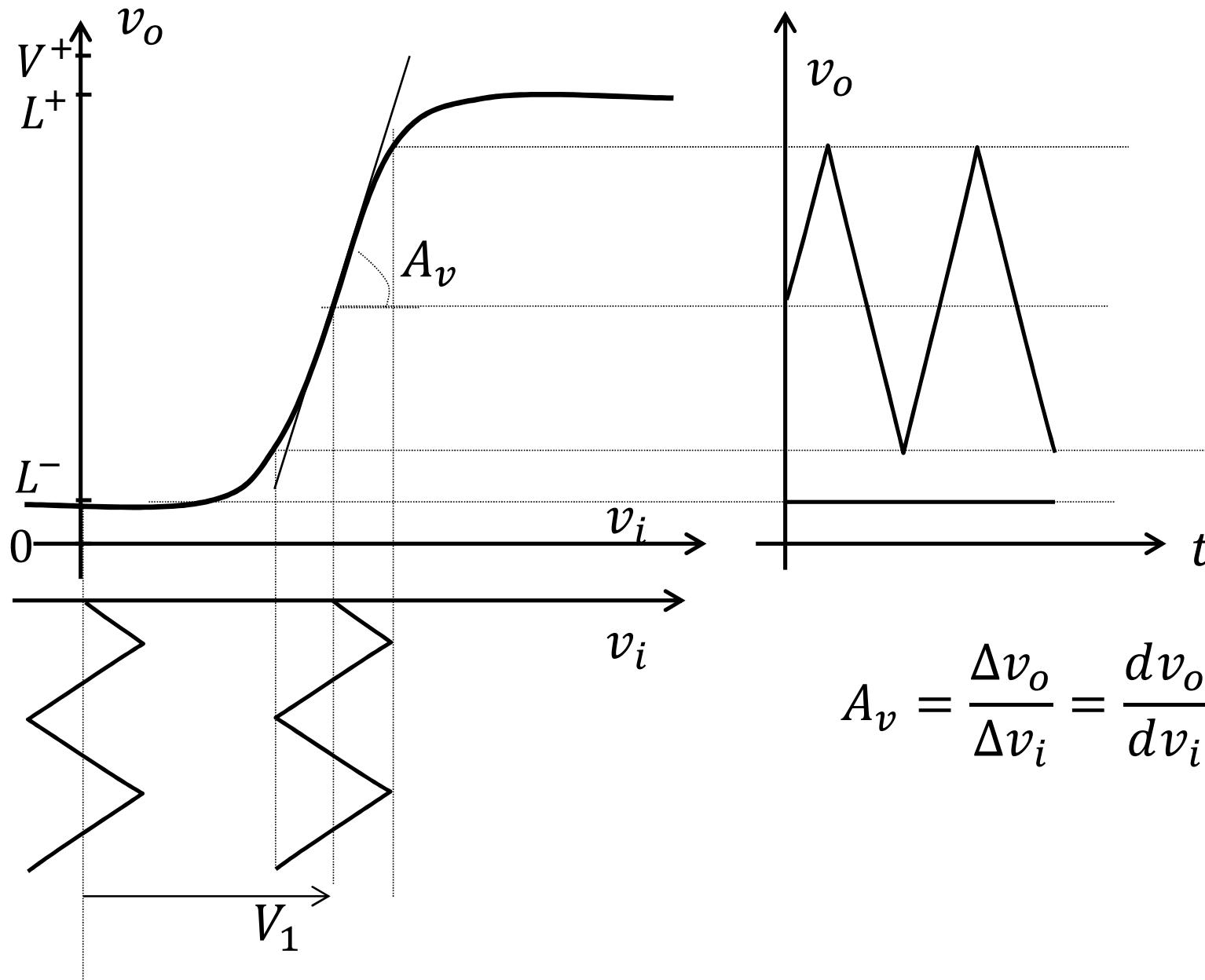
$$A_v = \frac{\Delta v_o}{\Delta v_i} = \left. \frac{dv_o}{dv_i} \right|_{Q \text{ bias point}}$$
