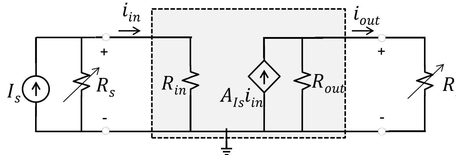
Short circuit:  $R_L = 0 \rightarrow \frac{i_{out}}{i_{in}} = A_{Is} \quad \left[ \frac{A}{A} \right]$  short circuit current gain
