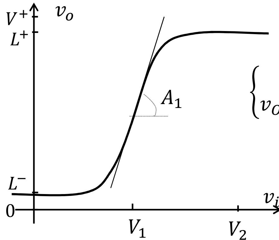
$$\begin{cases} v_{IN} = V_I + v_i(t) \\ v_{OUT} = V_O + A_v v_i(t) \end{cases}$$
