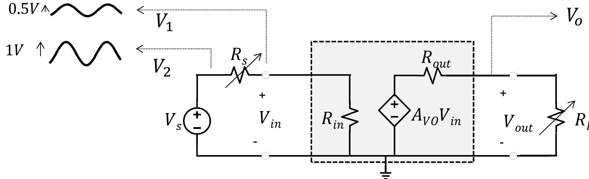
$$R_s = 1k\Omega \rightarrow \frac{V_1}{V_2} = \frac{R_{in}}{R_{in} + 1k}$$
