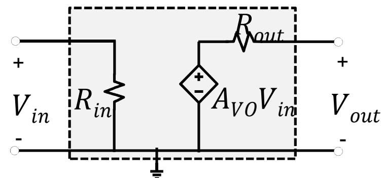
$$A_{VO} = \frac{V_{out}}{V_{in}} \Big|_{i_{out}=0}$$
