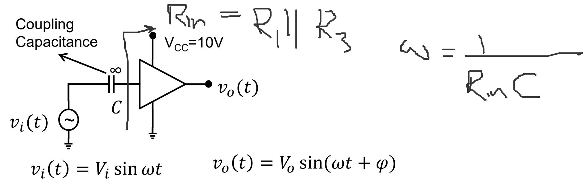
Transfer Function:  $T(\omega) = \frac{v_o}{v_i}$
