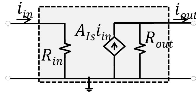
$$A_{IS} = \frac{i_{out}}{i_{in}} \Big|_{V_{out}=0}$$
