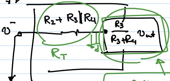
$$A_v = \frac{V_{out}}{V_{in}} = -\frac{R_3}{R_1} \times \frac{R_1 + R_2 + R_3 || R_4}{R_2 + R_3 || R_4}$$
