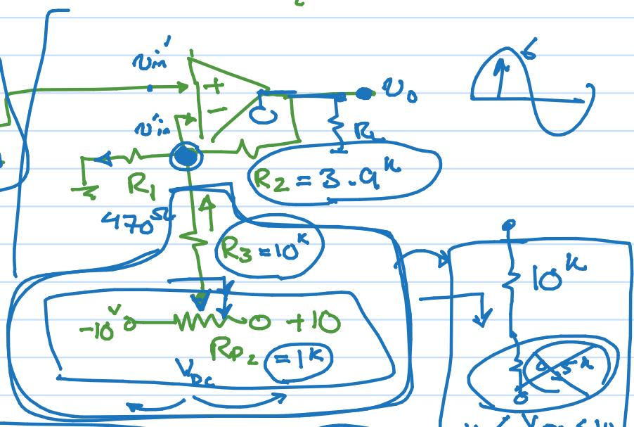
$$V_o = V_{in}' \left( 1 + \frac{R_2}{R_1} + \frac{R_2}{R_3} \right) - V_{DC} \frac{R_2}{R_3}$$
