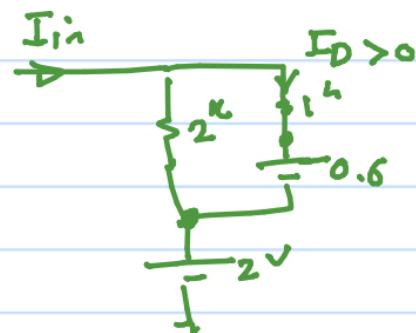
$$I_{1,h} = \frac{V_{i,n} - 2}{2 \text{ k}} + \frac{V_{i,n} - 2.6}{1 \text{ k}}$$
