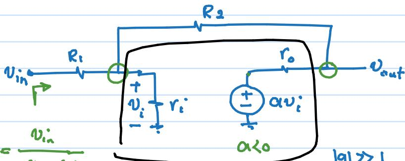
$$\left. \begin{aligned} & \frac{V_i}{r_i} + \frac{V_i - V_{out}}{R_2} + \frac{V_i - V_{in}}{R_1} = 0 \\ & \frac{V_{out} - \alpha V_i}{r_o} + \frac{V_{out} - V_i}{R_2} = 0 \rightarrow V_{out} \left( \frac{1}{r_o} + \frac{1}{R_2} \right) = V_i \left( \frac{1}{R_1} + \frac{\alpha}{r_o} \right) \end{aligned} \right\}$$
