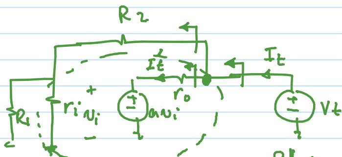
$$V_i = \frac{R_1 \parallel r_i}{R_1 \parallel r_i + R_2} V_t$$
